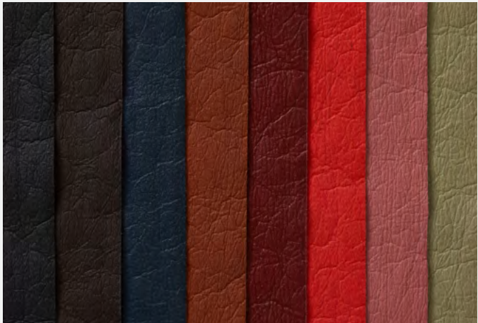
8. The Piñafelt® is coloured with pigments and coated to make Piñatex®
