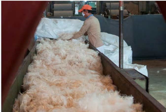
6. Fibres are purified and blended with polylactic acid (PLA) from corn
