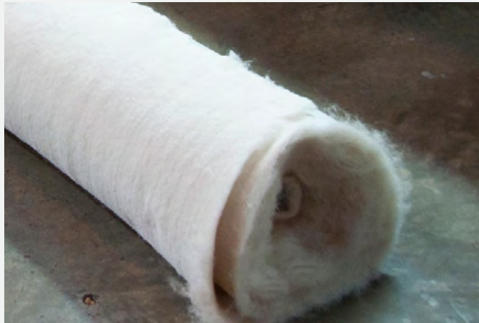
7. 80% pineapple leaf fibres mixed with 20% PLA makes the non-woven base called Piñafelt®
